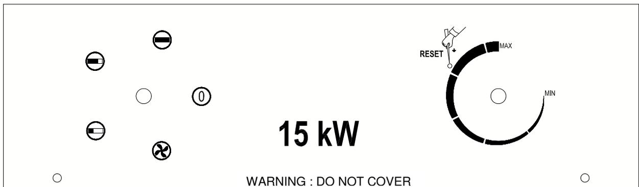
Three four and five positions rotary switch, which can be turned from 0 to 360 degree clockwise or counter clockwise, the first level is ventilator only, the second level is 5KW, the third level is 10KW and the four level is full power input. You can adjust the level clockwise or reverse.
